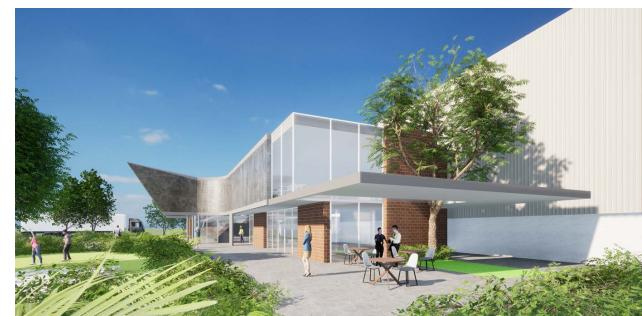
**Figure 160** Rendered impression of a potential landscape strategy that integrates trees and ground cover with built form to provide shade to paved areas around building, which then absorb less heat.
